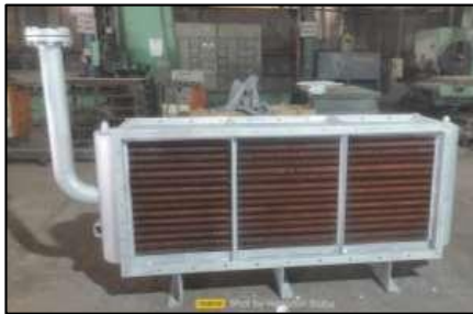
HEAT EXCHNGR,STEM TO AIR,420000 KCAHR - Fin Tube
