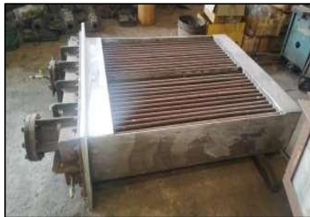
CU HEAT EXCHANGER
