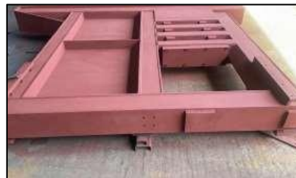
Charging Trestle for SCP Machine
