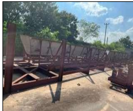
30mtr Conveyor with SS Slides
