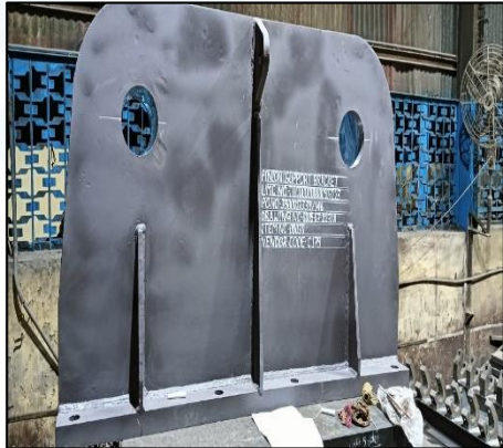
TGS PINION SUPPORT OF CRANE
