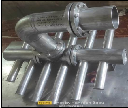
Distribution Tube - Coke Plant, Material Titanium
