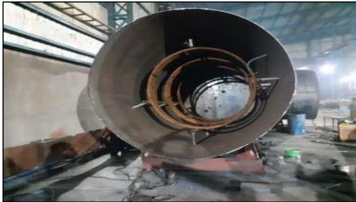
OPEN BOILER WITH COIL
