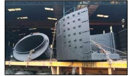
Stone Box - Conveyor Side
