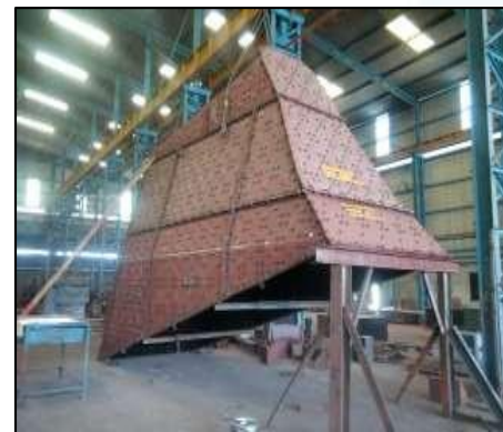
CHUTE WITH LINER
