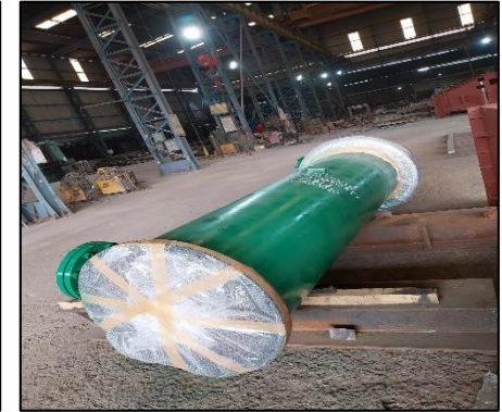
Heat Exchanger - VRTCF Vertical Shell & Tube Type Heat Load - 2265KW
