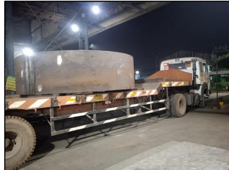
Shell For Rolling - 28mm X 1mtr X 12mtr - In DRA Unit - TSLP
