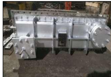
CU HEAT EXCHANGER
